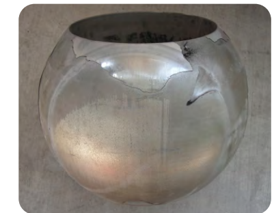
兖矿国泰锁渣阀维修
