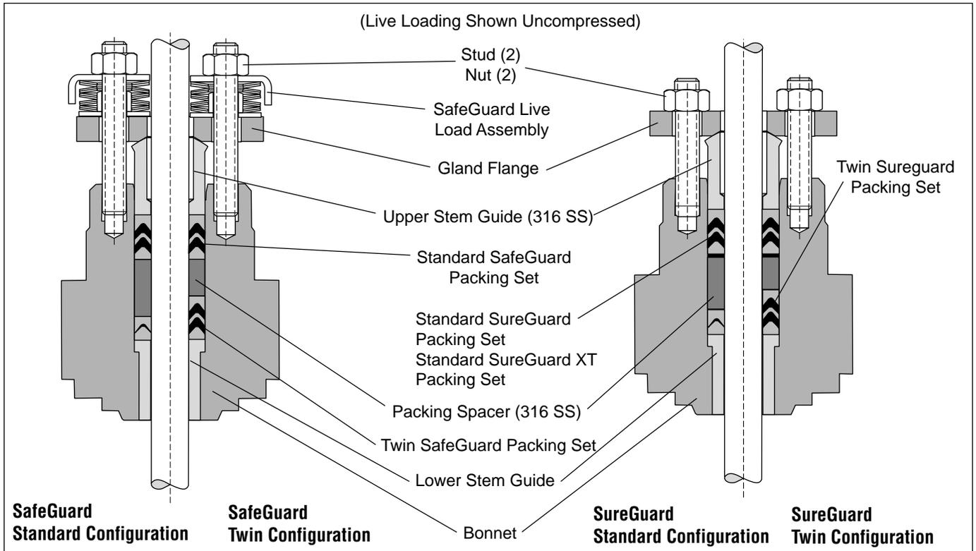
**Figure 20: SafeGuard Configurations for Valtek 2000**
