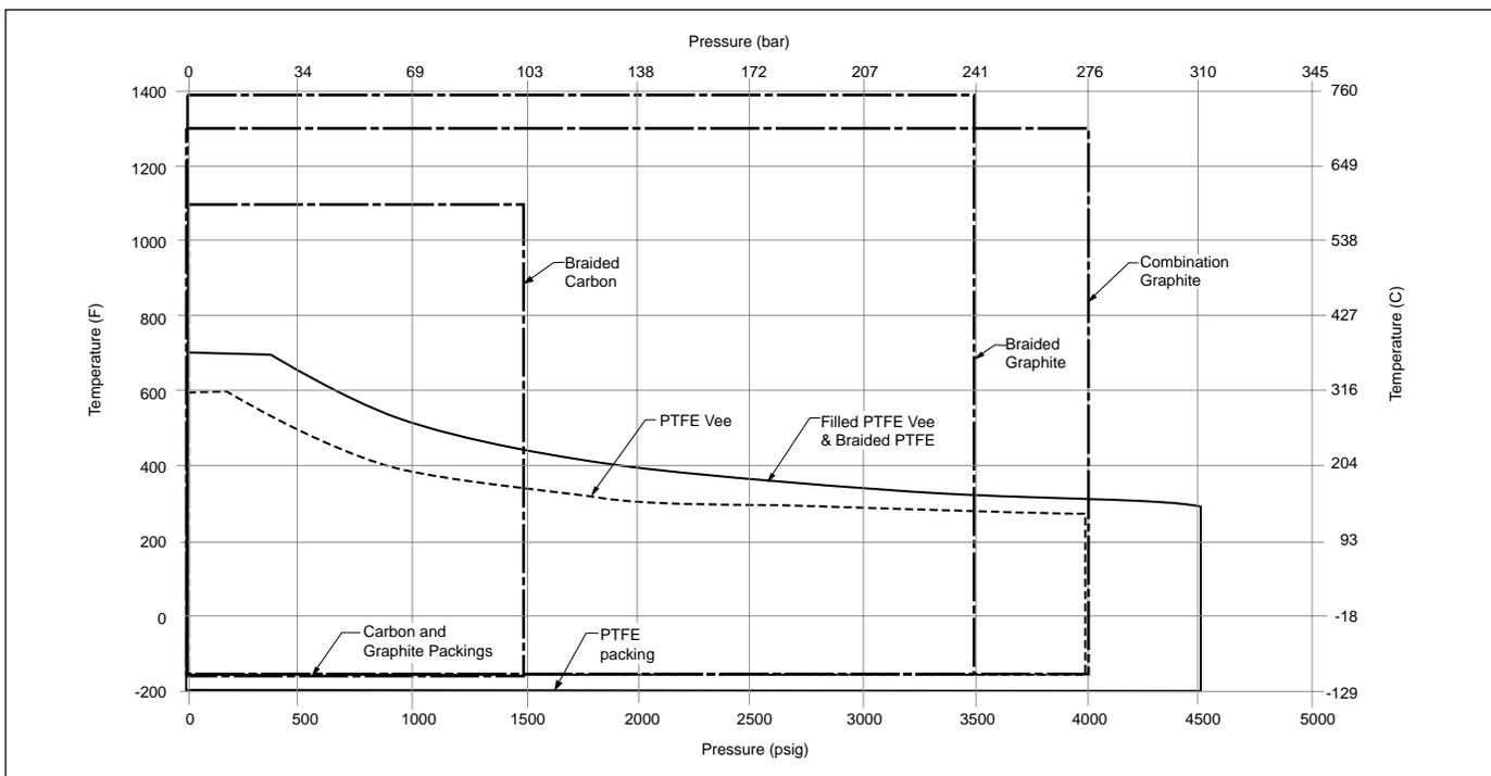
**Figure 23: Non-environmental Packing - Temperature and Pressure Guidelines - Extended Packing Bore**
