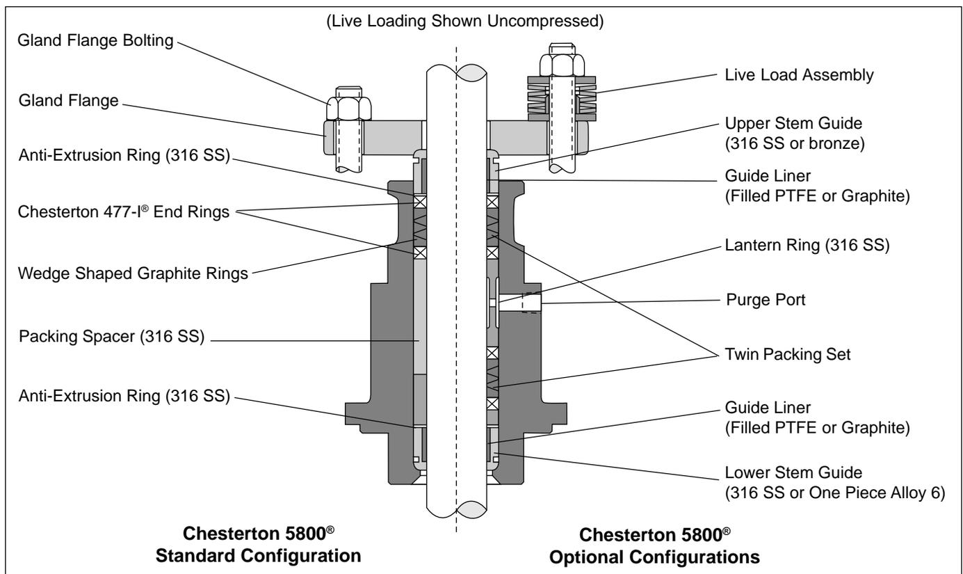
Figure 19: Chesterton 5800<sup>®</sup> Standard and Optional Configurations
