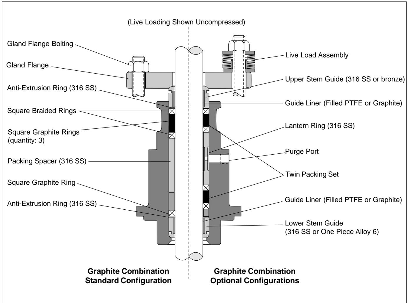
**Figure 31: Combination Graphite Packing System**
