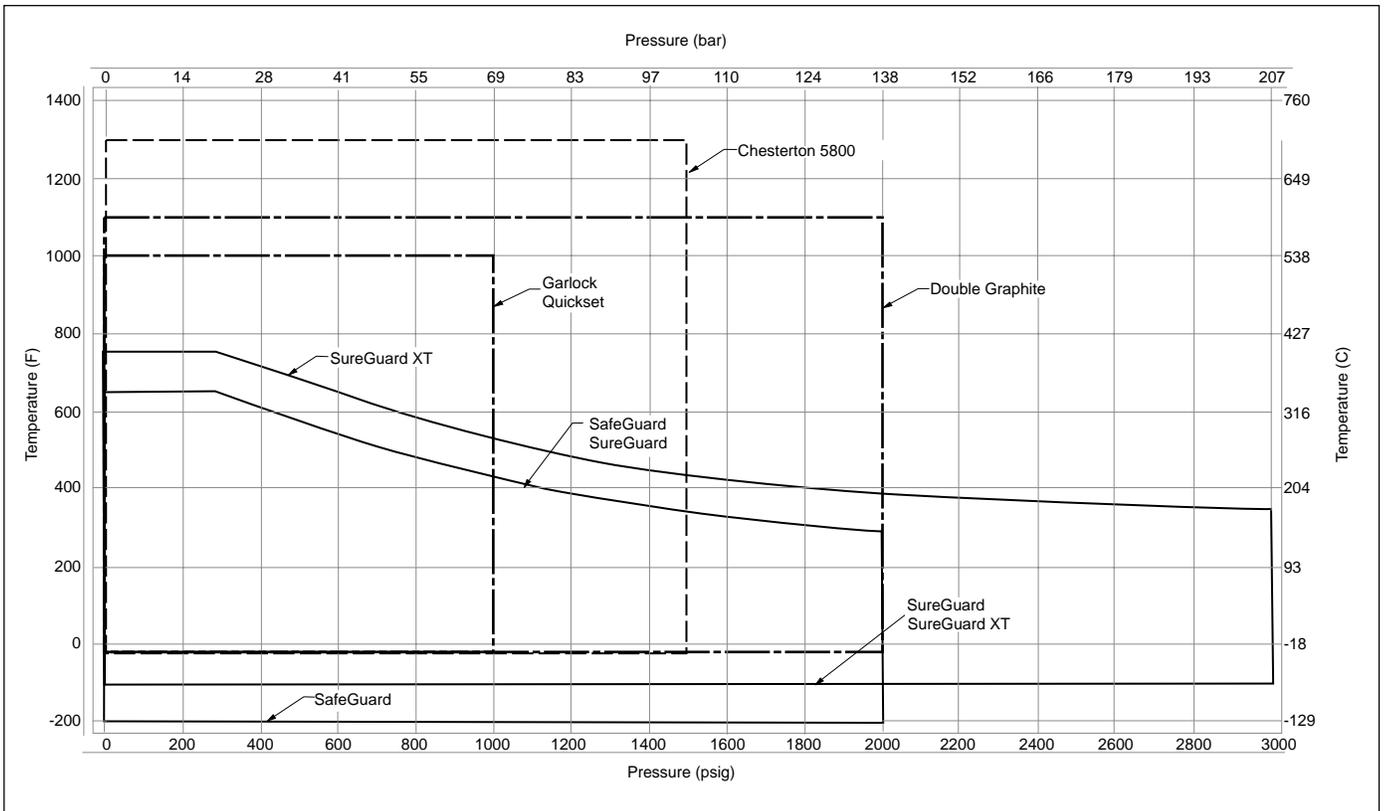
**Figure 13: Environmental Packing - Temperature and Pressure Guidelines - Extended Packing Bore**
