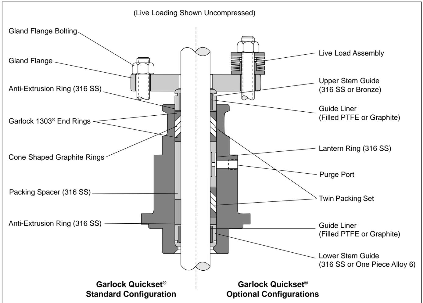
Figure 18: Garlock 9001® QuickSet Standard and Optional Configurations
