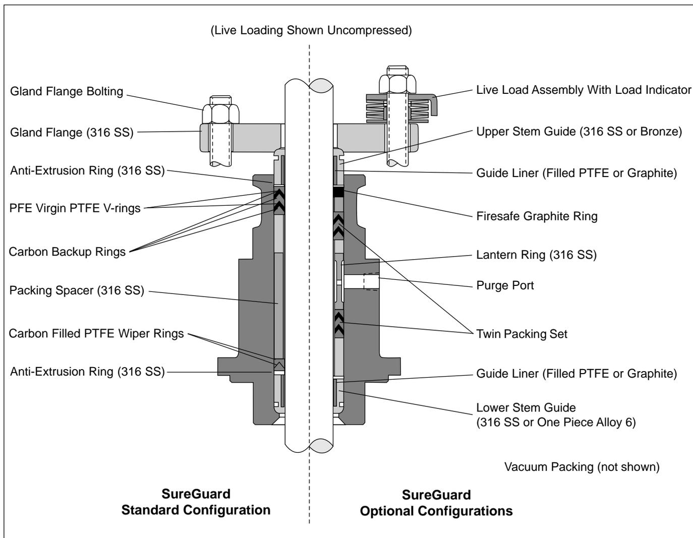
Figure 15: SureGuard Standard and Optional Configurations
