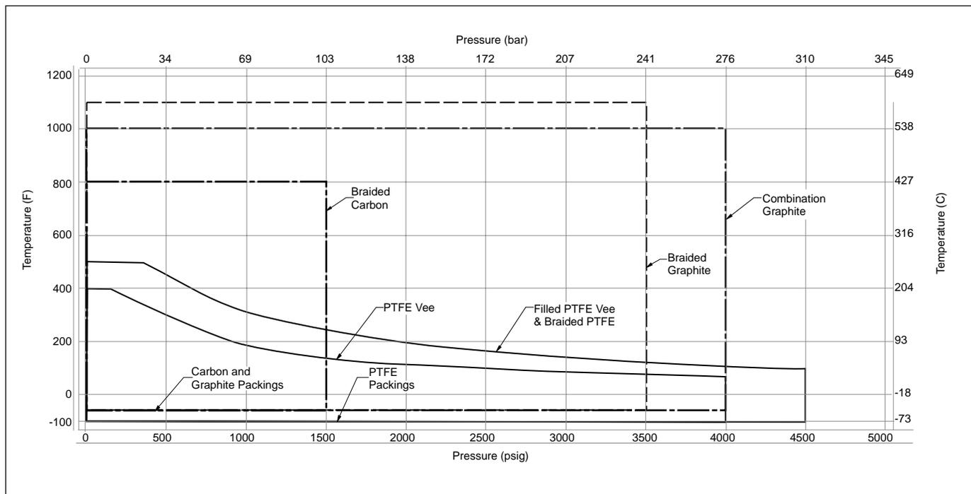
**Figure 22: Non-environmental Packing - Temperature and Pressure Guidelines - Standard Packing Bore**
