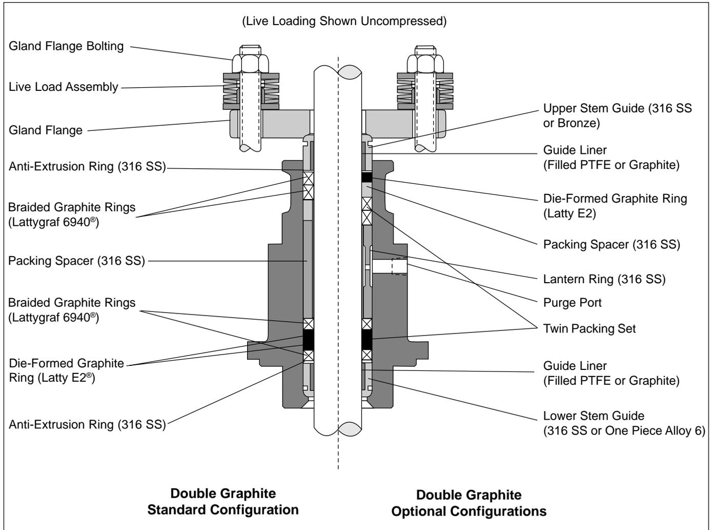
Figure 17: Double Graphite Standard and Optional Configurations
