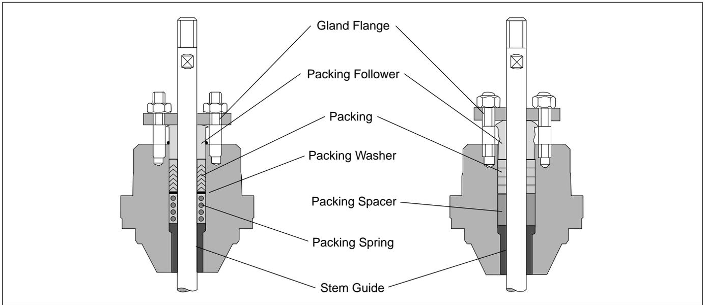
**Figure 32: Valtek 2000 with PTFE V-ring Self-adjusting Packing System**
