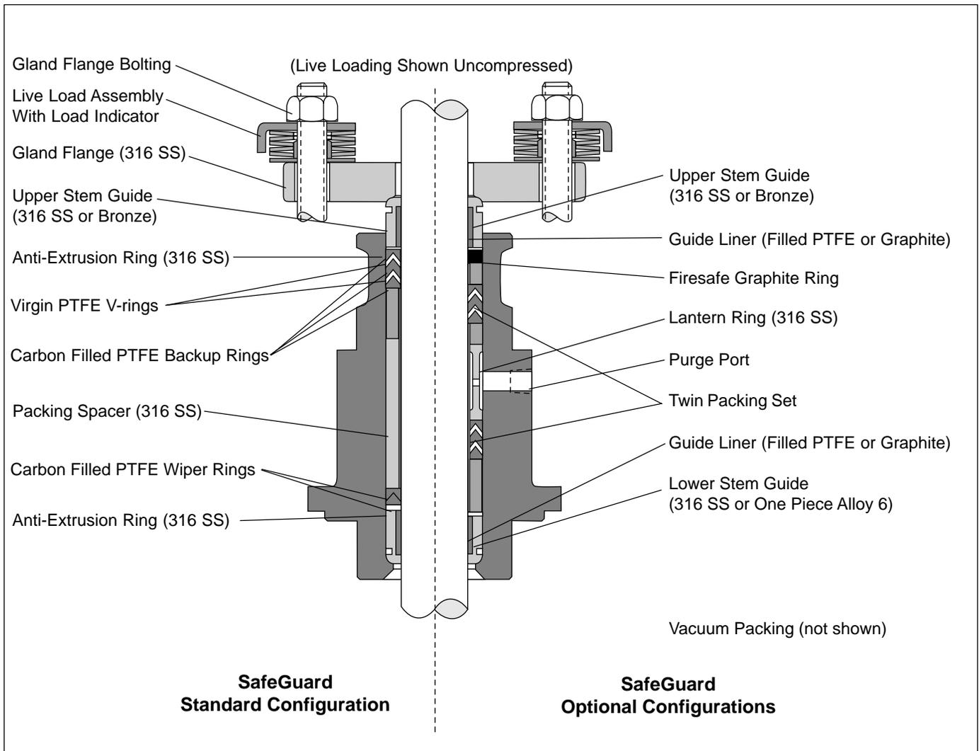
Figure 14: SafeGuard Standard and Optional Configurations
