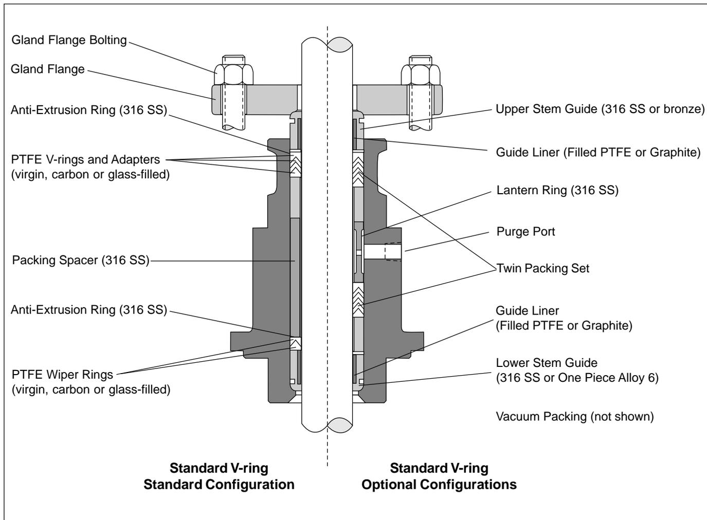
Figure 29: Standard V-ring - Standard and Optional Configurations
