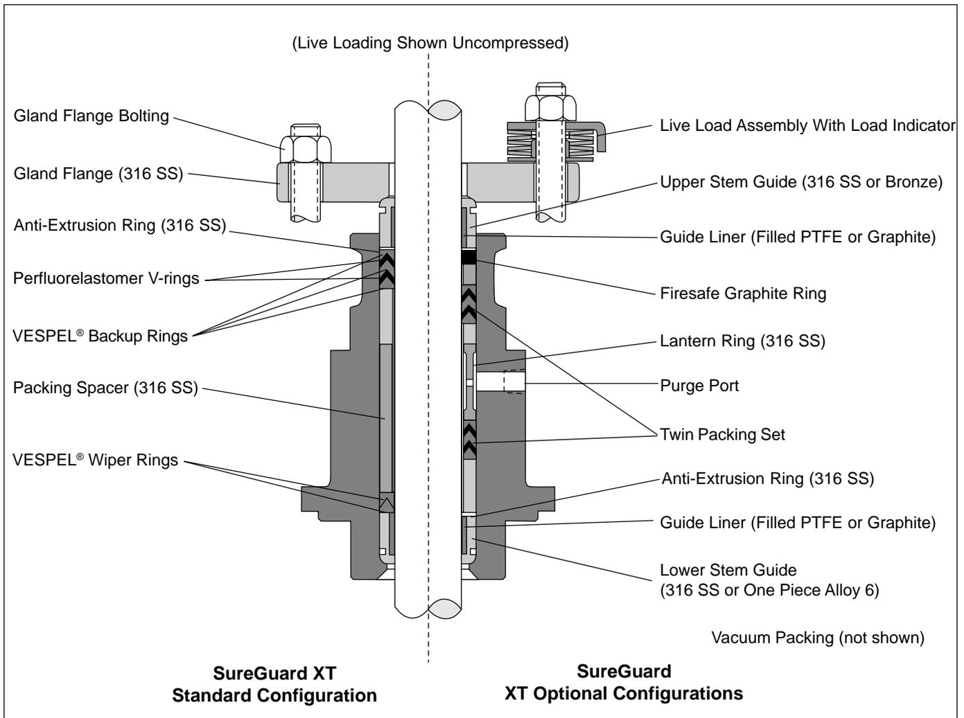
Figure 16: SureGuard XT Standard and Optional Configurations
