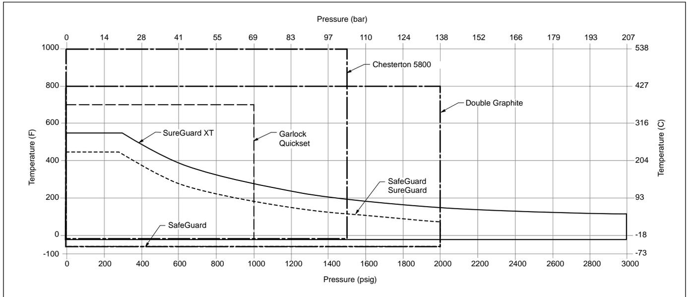
**Figure 12: Environmental Packing - Temperature and Pressure Guidelines - Standard Packing Bore**
